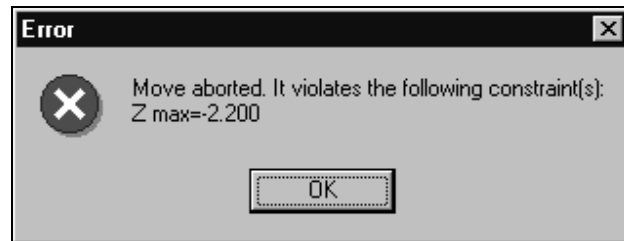
Figure 25-9. Example of a Manual Control error because the Biomek FX tried to move the pod too far on the Z axis
