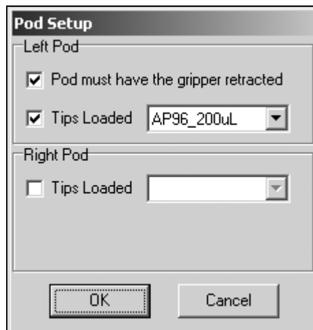
Figure 15-3. Pod Setup prompt for dual-pod Biomek FX instrument
