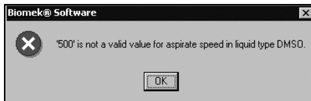
Figure 25-1. Example of a configuration error generated due to a Liquid Type Editor configuration problem
